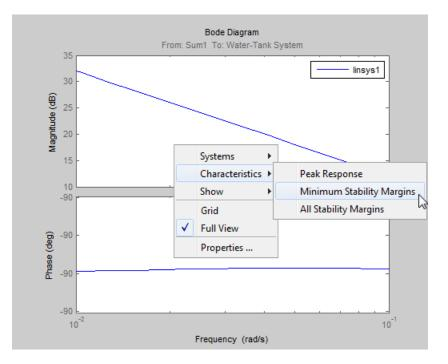
The Bode plot displays the phase margin marker. Click the marker to show a data tip that contains the phase margin value.
