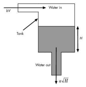
Water enters the tank from the top at a rate proportional to the voltage, V, applied to the pump. The water leaves through an opening in the tank base at a rate that is proportional to the square root of the water height, H, in the tank. The presence of the square root in the water flow rate results in a nonlinear plant.
