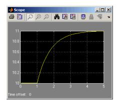
This action updates the Scope window with the response of the nonlinear model with the compensator design. This simulation shows that the rise time is less than 5 seconds and there is minimal overshoot. Thus, this compensator design meets the requirements of less than 5% overshoot and less than 5 second rise time.
